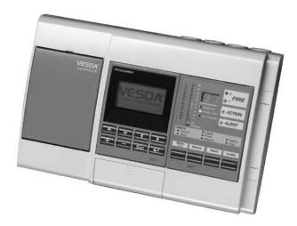
The LaserPLUS detector is the central element of the VESDA smoke detection product range. Using unique detection principles, the LaserPLUS has an alarm sensitivity range of 0.005%–20% obscuration/m (0.0015%–6.25% obscuration/ft). The LaserPLUS is classed as a "Very Early Warning Smoke Detector" which means that it detects fire at the earliest possible stage and reliably measures very low to extremely high concentrations of smoke.
