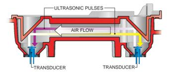
In this application, the ultrasonic flow sensing technology was adapted to monitor air rather than fluids. Two transducers (Blue) are used to continually send signals to each other. One signal travels with the flow (Violet), the other against (Yellow). The time difference between the two signals is used to calculate the rate of airflow within the pipe.
