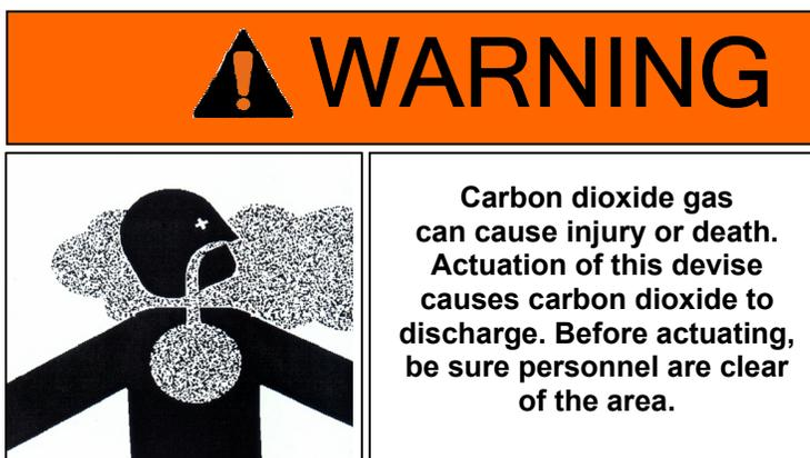
**4.3.3.1.1\*** Visual and audible devices shall be located at the entrance to each occupiable space protected by a CO<sub>2</sub> system and at the entrance to each space where CO<sub>2</sub> could migrate, creating a hazard to personnel. Provisions shall be made to prohibit entry of unprotected personnel . . . Persons who are not properly trained in the use of and equipped with SCBA shall not remain in spaces where concentration exceeds 4%.
